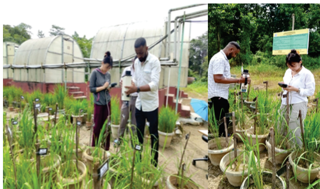
Fig. 2. Handling of hyperspectral radiometer/hyperspectral instrument in field condition
